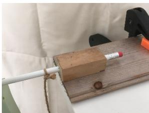
This image shows the drilled holding jig clamped to a table.
